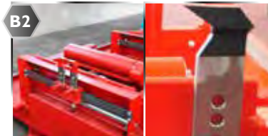
grip with two cylinders + mechanical grip lift
