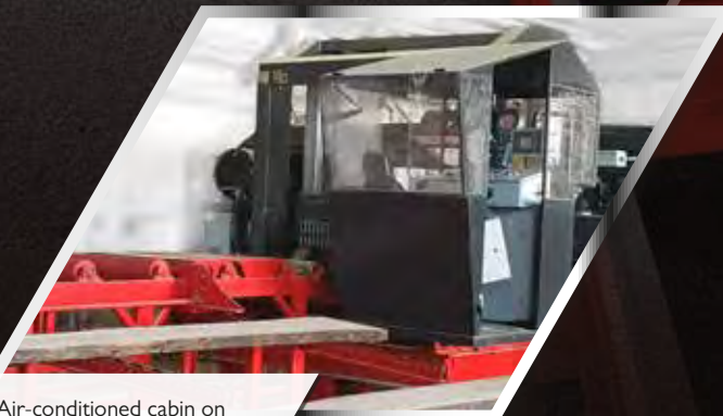
Air-conditioned cabin on the sawmill.
