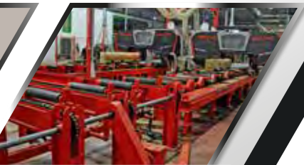
Machine can operate independently or connected in multi-line with several veneer bandsaws
