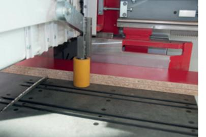
Because boards are cut to size and mitre cuts are performed simultaneously on only one machine, there is no need for handling from one saw to the next. This significantly reduces the risk of errors and damage.
