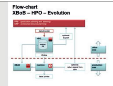
The operating data reporting of the MCS Evolution logs all relevant operating data, such as operating hours and the travel paths of the saw unit, feeder, pressure beam, etc. In addition, the running data of
