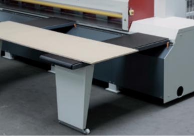
Three air flotation tables make panels and parts extremely easy to handle. Furthermore, all air flotation tables (except on the angle end stop) can be moved, which ensures good accessibility in every situation. In addition, the right table can be shifted to the outer edge of the machine, which opens up more space for comfortable positioning of, e.g., longer parts.
