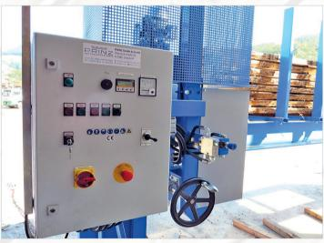
The Mobilcut Comfort+ offers automatic positioning via a length measuring system.
