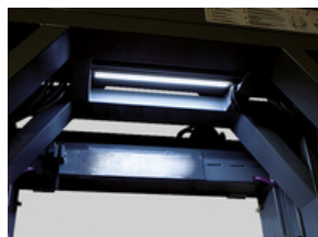
LED lighting (11 W)
