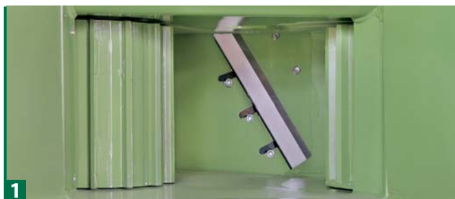
Detail of the material feeding mouth; the feeding rollers are visible on the base and, in the background, the disc with a chipping knife. Roller speed can be adjusted by the operator, in relation to the type of material to be chipped.
