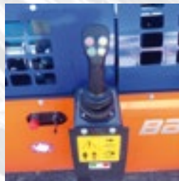
Ergonomic joystick control.
