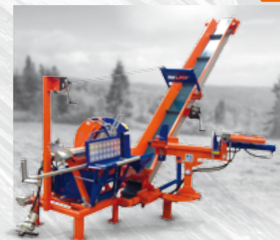
Drive motor mounted at the top of the conveyor for better grip on the belt
