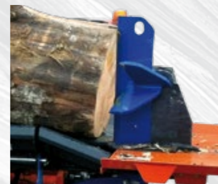
Hydraulic adjustable knife (available 2/4 or 2/6 way).
