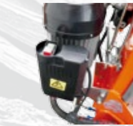
Power switch with thermal safety cut out.
