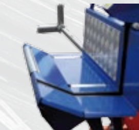
Rocking bench, with rollers for easy timber feeding and grip to avoid logs rolling while cutting.
