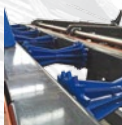
Infeed via powered toothed rollers for excellent grip even in the wet.
