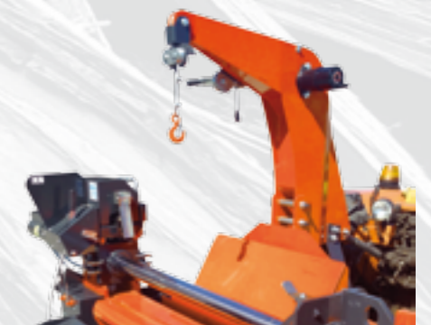
Optional 1 Ton winch with automatic unrolling device.
