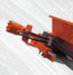
Drive motor mounted at the top of the conveyor for better grip on the belt
