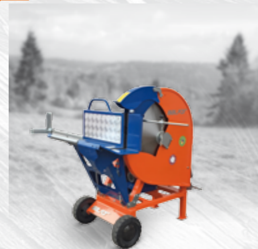
Rocking bench, with rollers for easy timber feeding and grip to avoid logs rolling while cutting.
