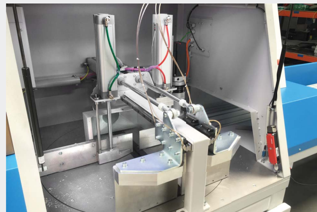
upper and side individually controlled clamps
