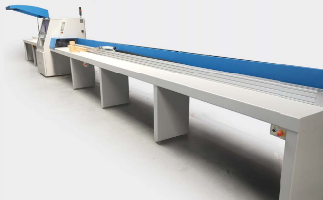
6 meters long infeed table with pusher
