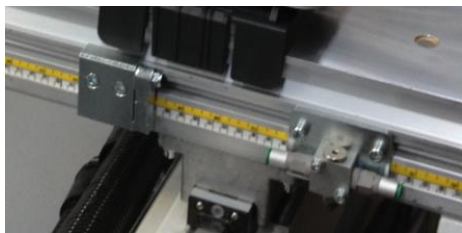
Kit for prearrangement of working table with 6 aluminum bars to apply clamping devices for arches and straight components
